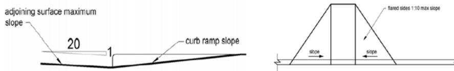
Figure 11: (1) Counter Slope of Surfaces Adjacent to Curb Ramp (2) Sides of Curb Ramps (Source: Department of Justice, "2010 ADA Standards for Accessible Design")
